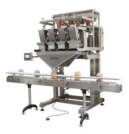
An automatic granular product weight filling machine that can be ordered with two filling channels that funnel into a single fill head, or four filling channels that funneled into two filling heads. Accutek vibratory feeders are the ideal solution for dry granular products that require precision weighing. The vibrating delivery channels that feed product to the load cells avoid damage normally encountered with feed screw or auger systems.
